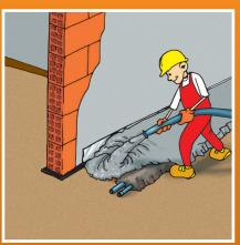
Apply FONOTEC PLUS by laying the rolls dry; lay a 10 cm rabbeted selvedge strip for overlapping at the sides. Whenever fluid or superfluid concrete screeds are used, the joints must be sealed with the appropriate adhesive tape PHONOTAPE ADHESIVE, in order to prevent percolation that may create sound "bridges" (this is not necessary in the version with adhesive selvedge).
